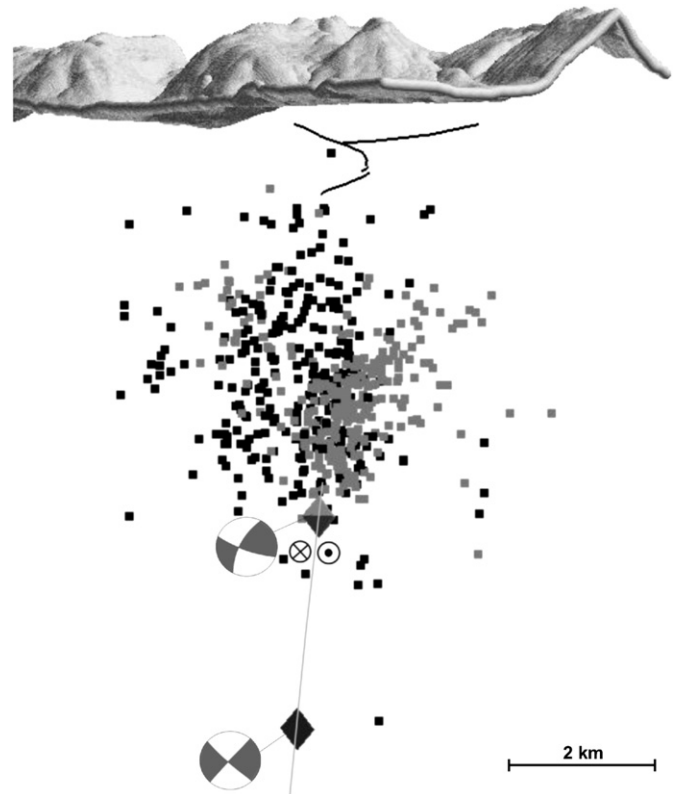
Fig. 10. Depth distribution of the 1998 and 2004 earthquake clusters. View towards the NW, perpendicular to the trend of Ravne fault zone. At epicentral depth the fault system is rupturing new, steep SW dipping planes, while in the upper part of the system, deformation is distributed along a wider zone. Strike-slip, oblique-slip and thrust events are distributed on NE and E dipping planes of the upper parts of the crust. Note, focal mechanisms are shown in plan view perspective.
